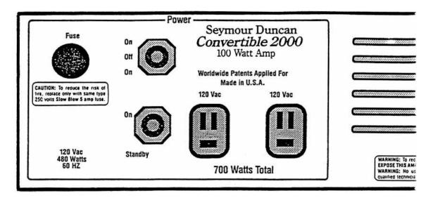
**1. Fuse Holder:** The fuse is located in the cap of the fuse holder. If the fuse fails, it must be replaced with one that provides proper current protection or you will void the warranty. The proper fuse rating for the 110-120 v. a c. *Convertible 2000 is 5A* 250V Slo Blow.
