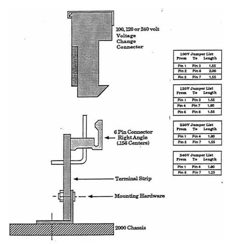
• WARNING: ALWAYS MAKE SURF, THE CONNECTOR ATTACHES TO THE TERMINAL STRIP AS SHOWN IN THE DRAWING ABOVE. FAILURE TO DO SO WILL VOID THE WARRANTY AND CAUSE ELECTRICAL FAILURE.
