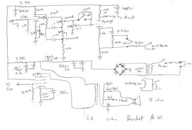
I just finished this schemo, that I assembled from the two incomplete schemos that are floating around. I own one of these, so I verified all the values and the complete schematic, as well as all the critical voltages, and the plate current. The Rocket A-10 is a single EL84 amp that sounds like a plexi at low volumes. It is mated to a celestion vintage 30. This amp is very loud for its size. Feel free to put this on your website.........JOe
