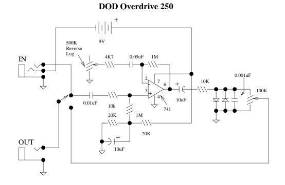
The DOD Overdrive 250 is Yet Another 741With Two Diodes On The Output. It is almost exactly the same as the MXR Distortion Plus, and a number of other units.
