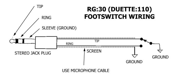
ENSURE THAT THE CHANNEL SELECTOR SWITCH ON THE AMPLIFIER IS SET TO THE 'CENTRE' OFF POSITION. OTHERWISE THE FOOTSWITCH WILL NOT WORK AS INTENDED.
