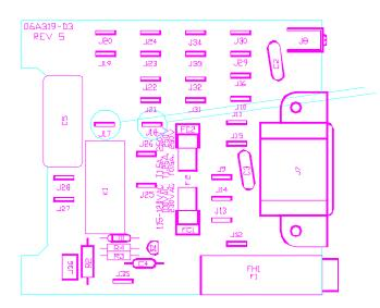
Add one 97-123-23 ICL assembly in series with J17 and the blue transformer lead and one in series with J18 and the gray transformer lead.
