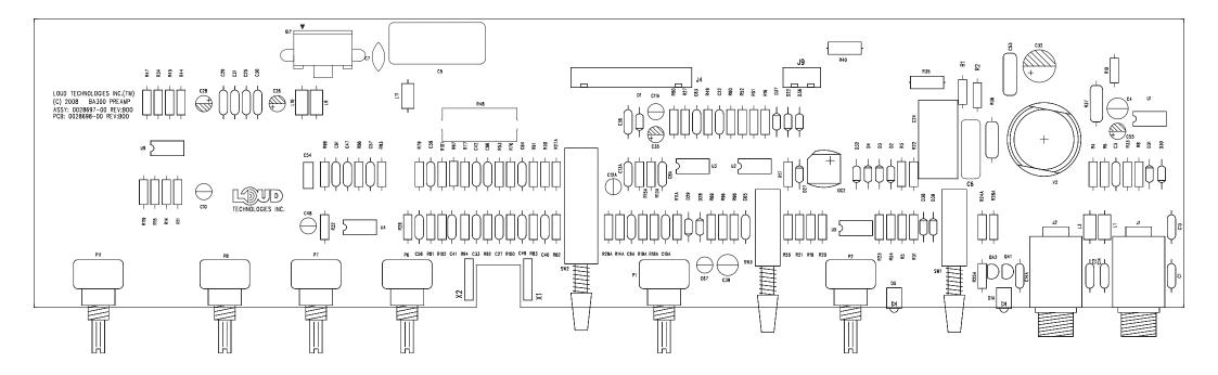
OVERALL FINISH THICKNESS: 1.6mm +/-.125mm DOUBLE SIDE PCB
